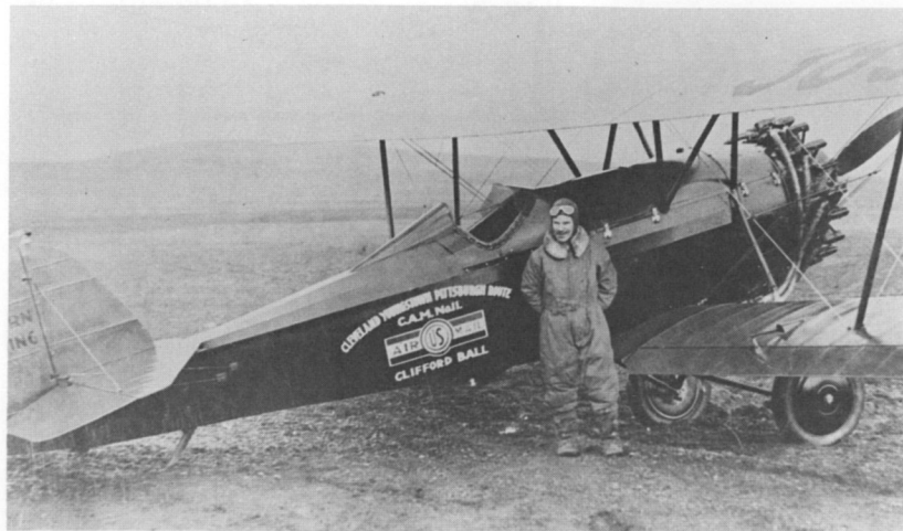
Pitcairn Mail Wing used for night Air Mail, 1928. 200 h.p., Wright J5 engine, 140 miles per hour, 700 lb. cargo. Dewey Noyes, pilot.
