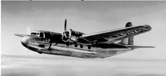
16/22 passenger civilian airliner, with a high wing And tricycle landing gear. Four examples were produced for KLM Airlines, and were used to
