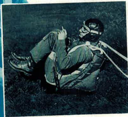
Man in position for Aerial Pick-Up. Body harness is attached to transfer loop suspended between ground poles.
