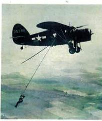
As crewman inside plane starts auto-matic reeling device, man is drawn up to plane. It's unnecessary for him to do any hand-over-hand climbing.
