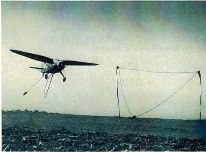
All American plane, Pick-Up arm down and incoming container trailing, approaches station.
