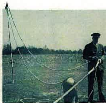
Transfer loop, attached to outgoing container, is strung over ends of poles by attendant.
