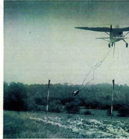
Out-going container trails behind plane as ship gains altitude. It is reeled in automatically.
