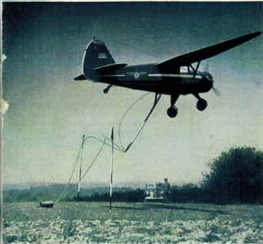
Climax of a perfect approach comes when hook at end of trailing arm engages transfer rope between station poles.
