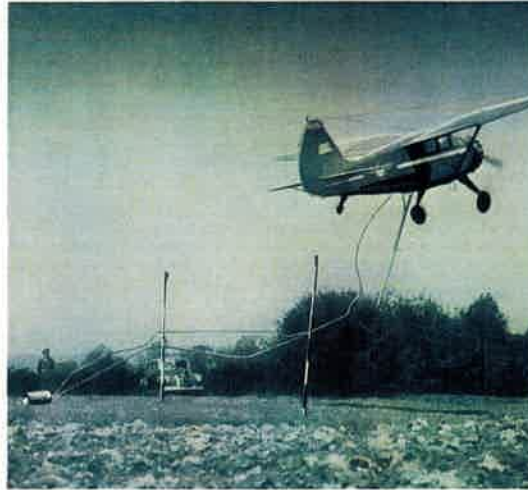
Container, cushioned against shock by rope's elasticity and Pick-Up mechanism, on its way as pilot begins climb.
