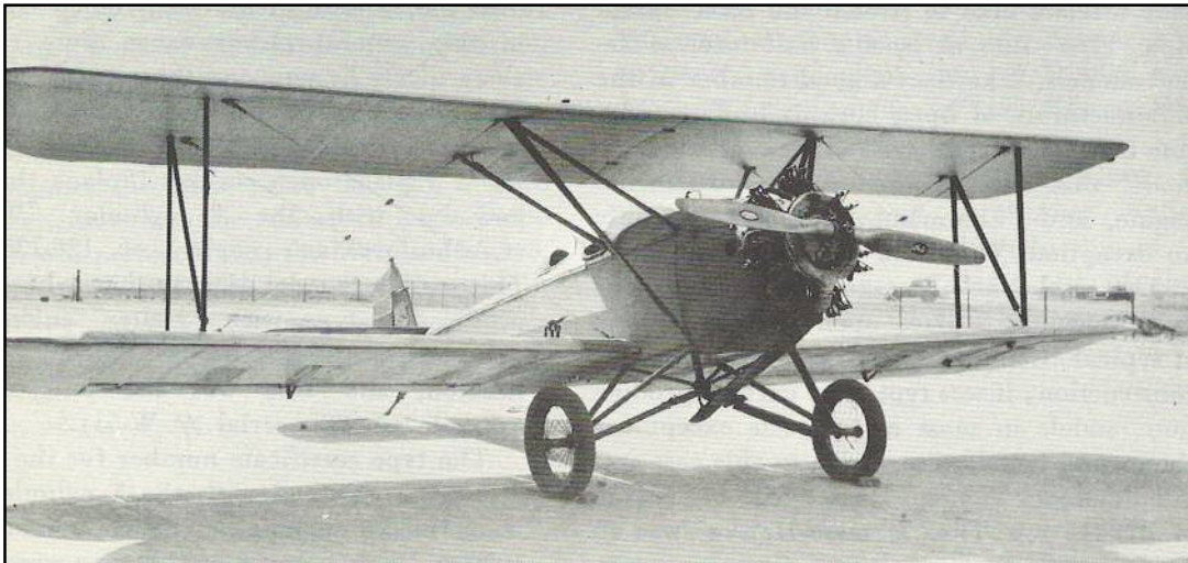
Wide landing gear is apparent in this photograph of a model 3C3-B. Wire wheels obviously have no brakes. Flying and landing wires are visible. The Command-Aire fact sheet indicates, "Front flying wires are the same size as employed on Douglas O-2 Army planes. Rear wires are one size smaller. Command-Aire equipped with OX-5 motor has a safety factor as great as found in army training ships of the PT-1 model. Pilot may rest assured ship is structurally equal to anything it may ever be called upon to do."
