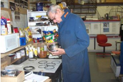
Deke Johnson inspecting and fitting rings on the pistons for the Challenger engine.
