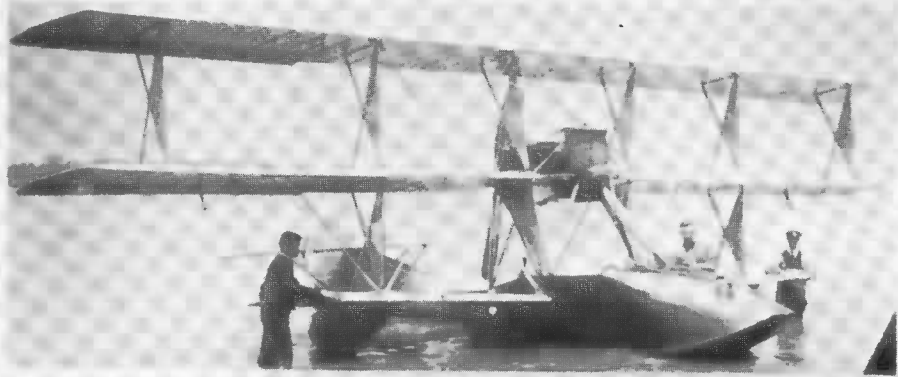
RIGHT: Rare photo. Curtiss "F" Triplane Flying Boat with OX5 engine. About 1915. (Photo from Geo. A. Page, Reynoldsburg, Ohio.)
