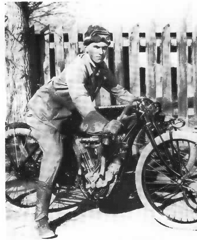
Art Goebel (1914) and his home built short coupled Indian racer (twin), equipped with Savannah high lift racing cams. Goebel won many Div. and track races.
