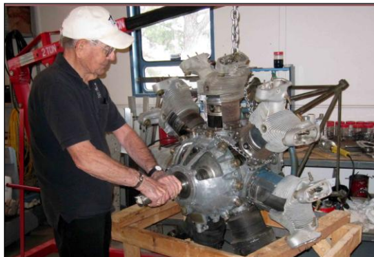
E. C. "Easy" Manny is building a cut-away radial engine for demonstration of the components and rotating operation of radial engines.
