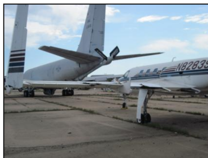
degrees from its original position. The airstair blew into the Beech Starship and damaged its flaps and ailerons.
