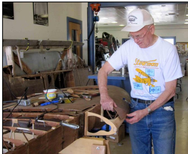
Stan Koehn works on the wing tip of the Beech Stagger Wing (Model 17) acquired by the museum.
