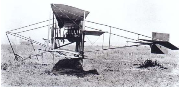
Curtiss E Military S.C. No. 6 – Note control seat cradle and steering wheel on the yoke.
