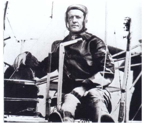
Lt. Foulois in Wright – Note telegraph key mounted on control stick, field radio mounted in seat. In flight transmissions, air to ground, were made to the Maneuver Div. in Texas.
