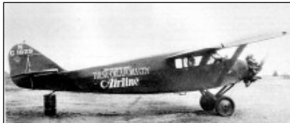
Stinson “Detroit” SM-1 (Pilot plus 4 passengers) Engine – Wright “Whirlwind” J5 220 h.p. Cruise - 105 mph Price - $12,000-$12,500
