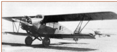
Buhl “Air Sedan” CA-5A (5-7 place) Engine – Pratt & Whitney “Hornett” 525 h.p. Cruise – 118 mph Price - $19,500
