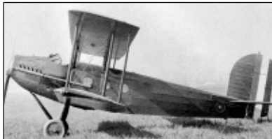
Douglas Transport C-1 (Two pilots, 6-8 passengers) Engine - “Liberty 12” 400-420 h.p. Cruise – 95-105 mph Price - $16,000 (Note open pilot cockpit)
