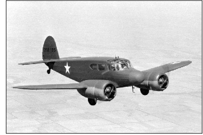
A Cessna A-17 "Bobcat" twin 245 h. p. Jacobs engines. Cruise 175 mph.
