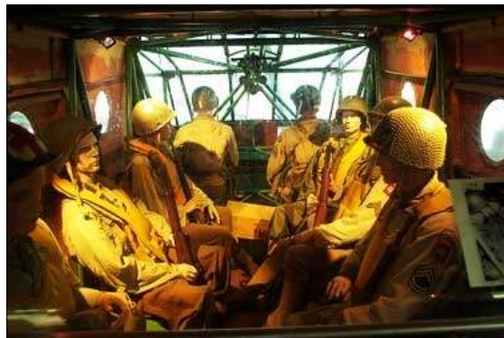
The glider was flown by two pilots, and carried thirteen armed troops
