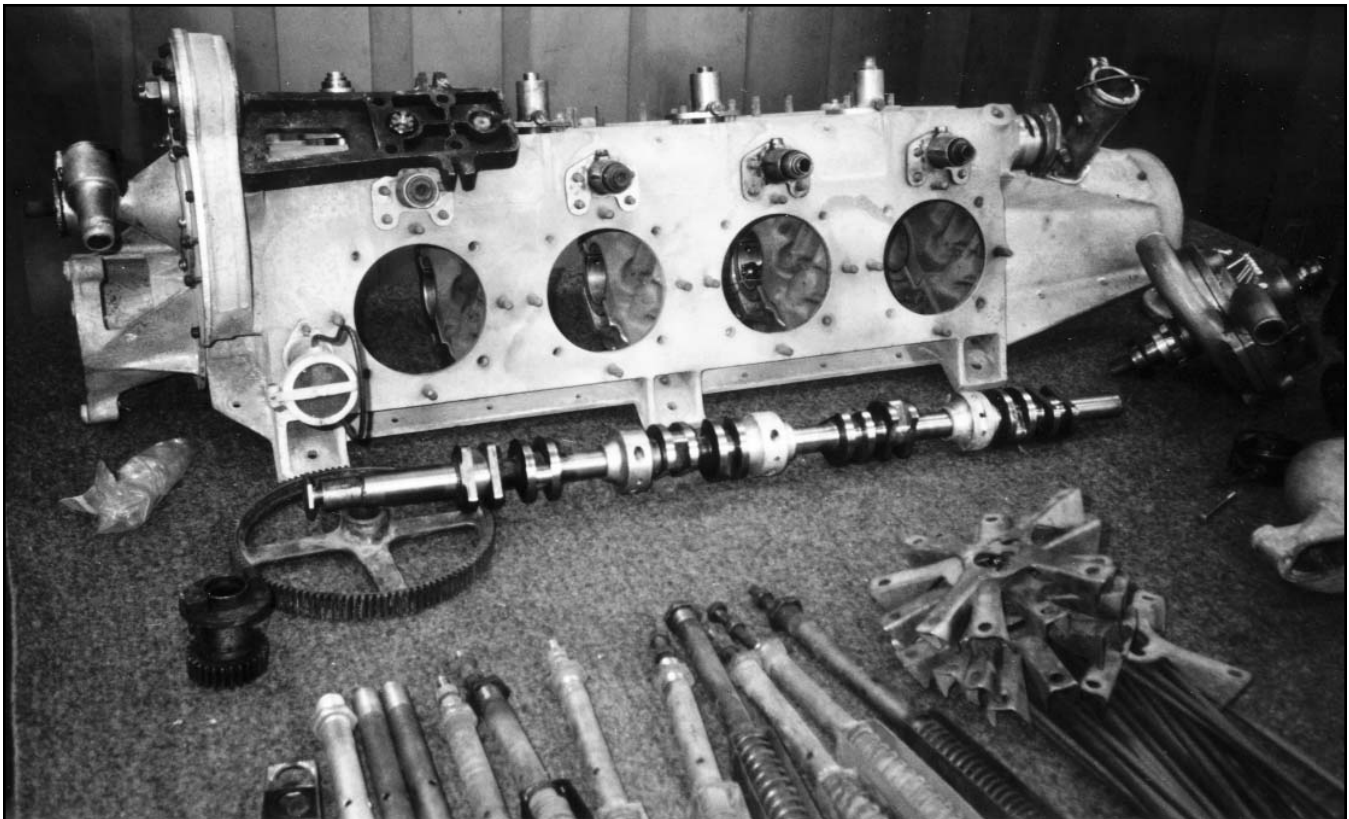
The direct drive crankcase is compact. Two rows of co-axial cam followers give an idea of the amount of stagger needed to take side by side rods. In front of the crankcase, the camshaft shows the eight exhaust cams, each flanked by a matched pair of inlet cams.
