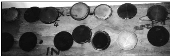
Valves removed for checking. Several show decked outer edges, a sure sign of inclined valves floating and touching.
