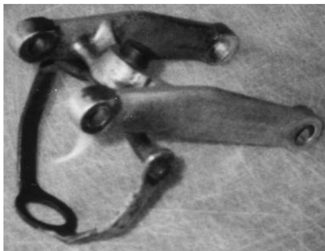
Inlet rockers, showing the Miller "Positive Action" valve yoke.
