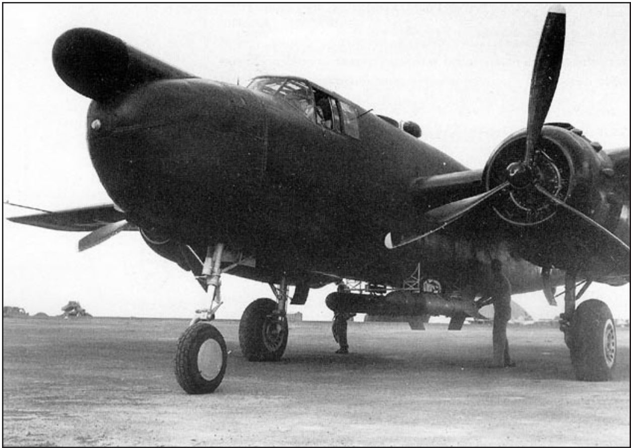
A North American PBJ of VMB-612 armed with Tiny Tim 11.75" rockets for night radar-assisted antishipping operations from Okinawa into the Japanese main islands and the Korean west coast (USMC)
